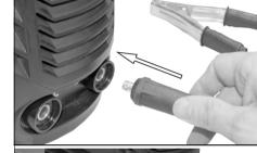
Welding rod holder lead to the (+) Positive terminal
