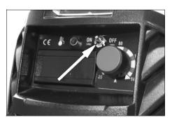
If you wish to turn off this feature, set the VRD switch on the front panel to OFF. We recommend that you leave it switched ON.
